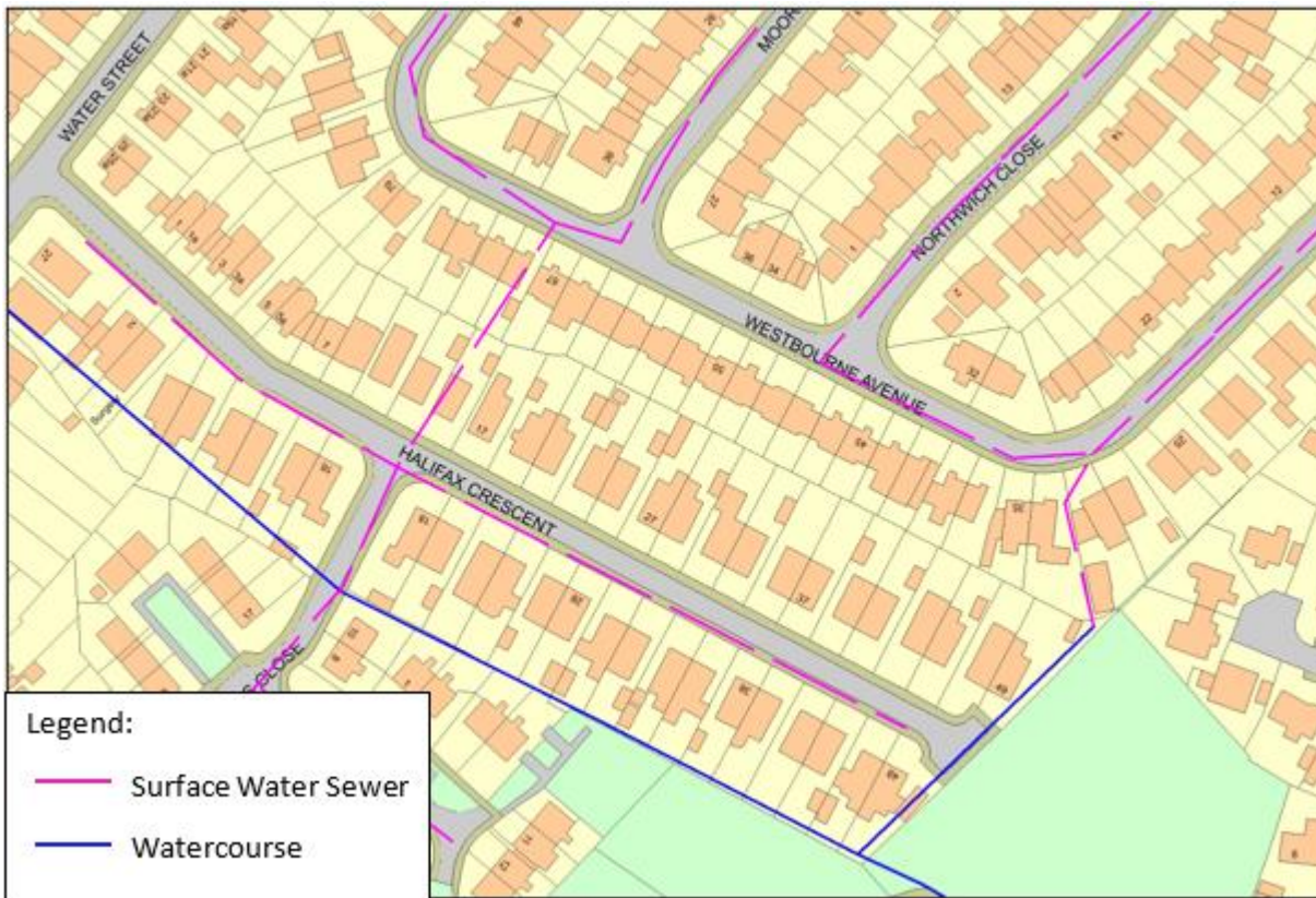
Figure 2 Surface water drainage network
